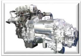
Integrated generator-motor power system (Range Extender)
