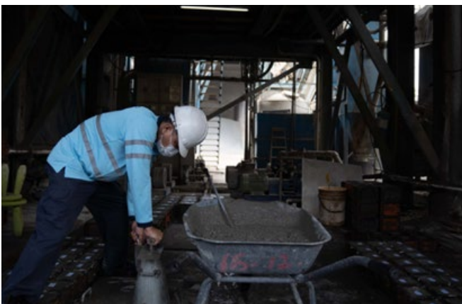
An Island Concrete employee doing slump check on the consistency of fresh concrete
