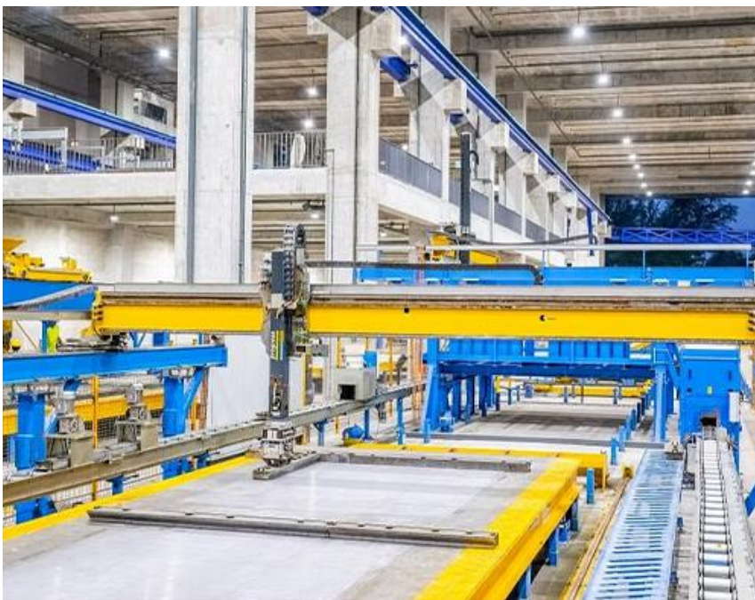
A close-up view of the automated concrete spreader at the HL-Sunway Prefab Hub, a new integrated construction and prefabrication hub by Hong Leong Asia and Sunway Construction.
